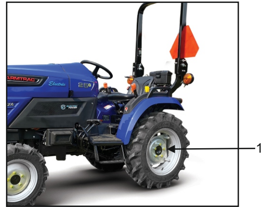
(1) Rear Wheel Bolt (Torque 245 To 270 N-m)
