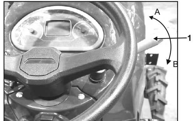
(1) Hand Throttle lever if (B) INCREASE" (A) DECREASE"
