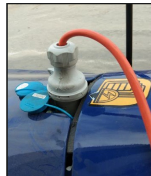
RCD Charging Cable Plugged In
