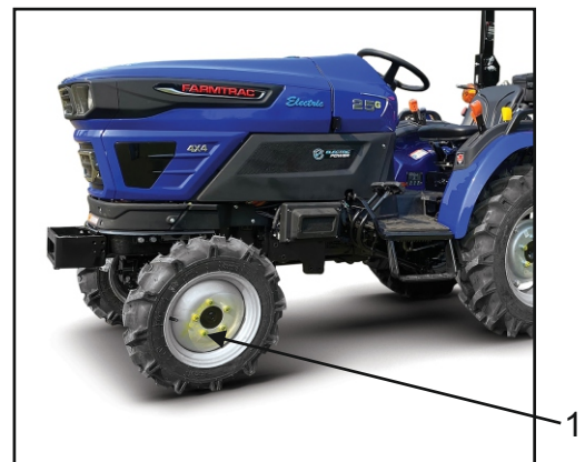
1. Front Wheel Bolt (Torque 110 to 130 N-m)
