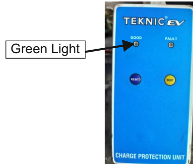
RCD – Residual Charge Device
