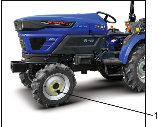
(1) Front Wheel Bolt (Torque 110 to 130 N-m)
