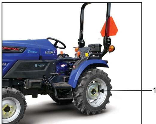
(1) Rear Wheel Bolt (Torque 245 To 270 N-m)
