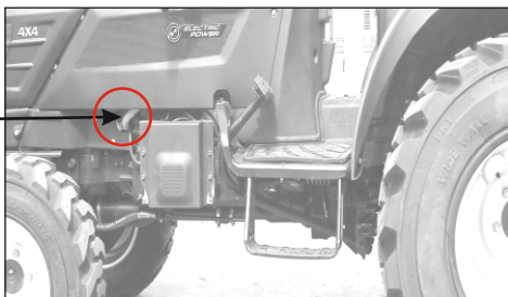
1. High Voltage Cable
